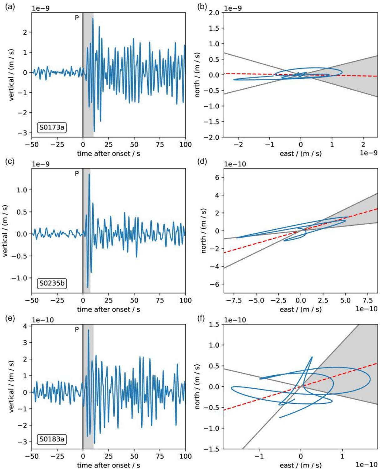
**Figure 9.** Vertical component VBB seismograms and horizontal particle motion for the three events with clearest polarization (S0173a, S0235b, S0183a). The red line on the particle motion plots indicates the azimuth chosen visually, the shaded gray area indicates the estimated uncertainty. Details on error determination methods are in Clinton et al. (2020).
