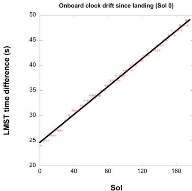
**Figure 4.** Drift in the Local Mean Solar Time due to the free-running onboard clock on InSight spacecraft. Here, the LMST time difference corresponds to the difference between the onboard time converted using WebGeocalc algorithm and Savoie et al. (2019) algorithm, expressed as integers. The data are plotted for 6 months from Sol 0 (November 26th, 2018). The dark line is fitted to the data, and corresponds to a linear increase of the drift of 0.139 s per sol.
